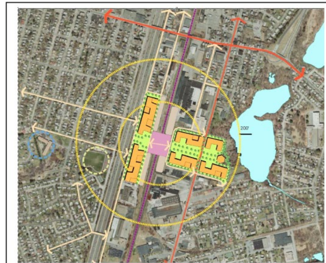
Figure 2-4 Wellington and Elmwood Avenues - TOD Option Light colored circles show 1/4 and 1/2 mile walking distances, light colored arrows show options for existing and new pedestrian/bike connections
